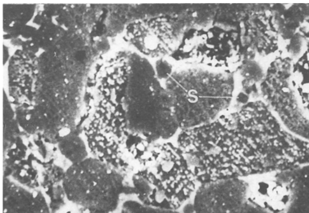
Figure 5 Scanning electron micrograph of Type B sample (bar = 10\ \mu\text{m} , S = spinel).
